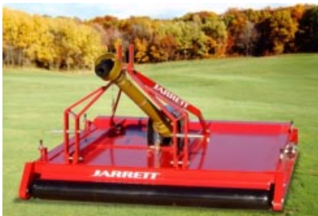
The HR150 roller slasher (left hand offset mounting)
